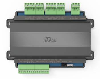
Driver board dimension: 179.5mm(L) x 116mm(W) x 50mm(H) ±1mm
