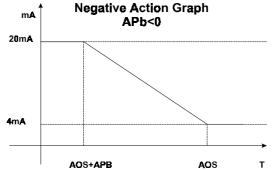
**NOTE**: When the defrost is in progress, the analogue output is set to the minimum value (4 mA). This condition lasts until defrost terminates.
