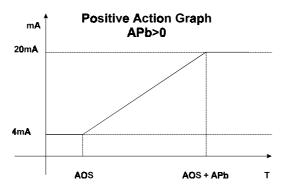
In the common area between AOS and AOS+APb the analogue output is:
