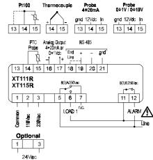
Pt100 with 2 wires: the terminals 13 and 14 must be shorted circuit.
