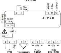
Power supply 24 Vac/dc: connect to the terminals 10-12 Pt100 with 2 wires: the terminals 2 and 3 must be shorted circuit
