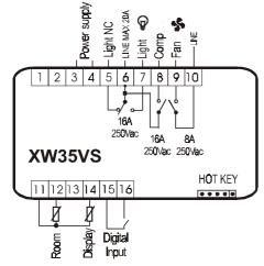
Power supply: use terminal 3-4; according to the model 230Vac or 120Vac or 24Vac
