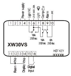
Power supply: use terminal 3-4; according to the model 230Vac or 120Vac or 24Vac
