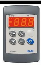
To display and modify target set point; in programming mode it selects a parameter or confirm an set operation
