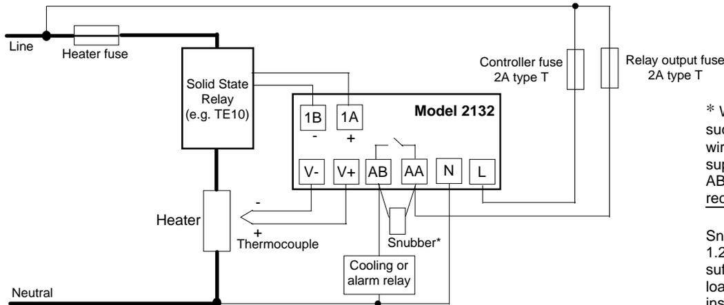
\* When switching inductive loads such as contactors or solenoid valves, wire the 22nF/100Ω 'snubber' supplied across relay terminals AA & AB. This will prolong contact life and reduce interference.
