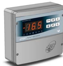
Fig. 3: close the front panel, making sure that all the wires are inside the box and that the box seal sits in its seat properly. Tighten the front panel using the 4 screws, making sure the O-rings on the head of each screw are used. Power up the panel and carry out thorough reading/programming of all the parameters.
