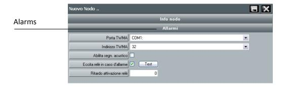
In this section TWMA module (if present) is being configurated for the alarm relay activation
