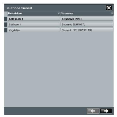
Select the device which history analysis is needed (it's possible to select up to 4 instruments at the same time, in case a comparision is requested).
